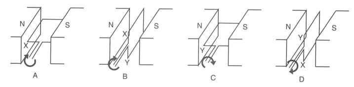
The diagram above shows a reduced scale model generator in which the side length of the loop is 50 cm and the magnets produce a uniform field of strength 1.2 T between them.
