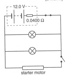
The starter motor of the car needs about 50 A to work effectively.
